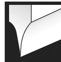
Conventional Hollow-Ground Edge
